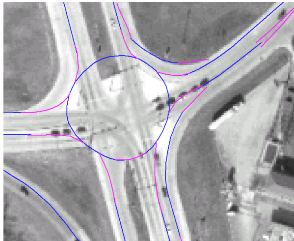
Figure 4 – Link-Connector Structure of Two-Lane Roundabouts
