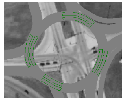
Figure 12 – Reduced Speed Zones for Two-Lane Roundabouts
