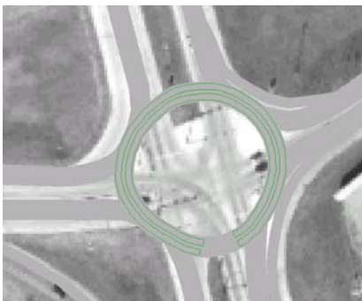
Figure 10 – An Incorrect Way to Code Reduced Speed Zones
